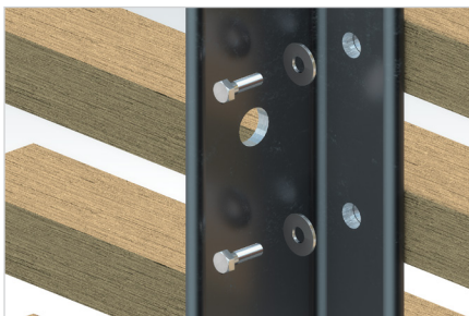
Installation of the supporting structure. The pre-drilled holes are wider (2 to 4 mm) than the bolt shaft to allow for expansion of the board. Washers are required as shown.
